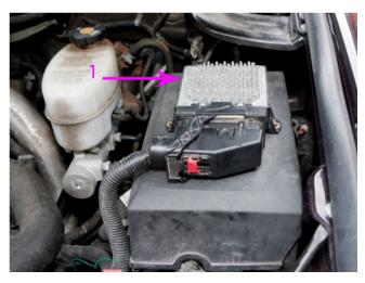
Important: DO NOT relocate the transmission control module (TCM) if aftermarket equipment HAS NOT been installed on the engine.
